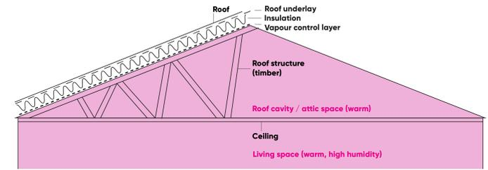
A warm roof has its insulation installed above the roof structure. This keeps the attic space and structure (timber or steel) warm. Therefore, the roof structure doesn't suffer through daily temperature fluctuations and subsequently prevents condensation as the surfaces remain warm.
