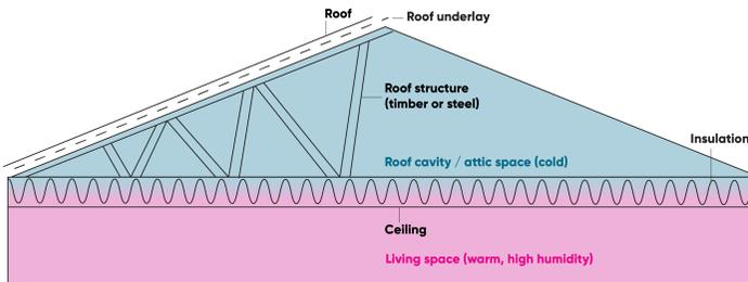
A cold roof means that insulation is installed at the ceiling line, keeping the house warm but the attic space cold. The majority of NZ houses have a cold roof.
