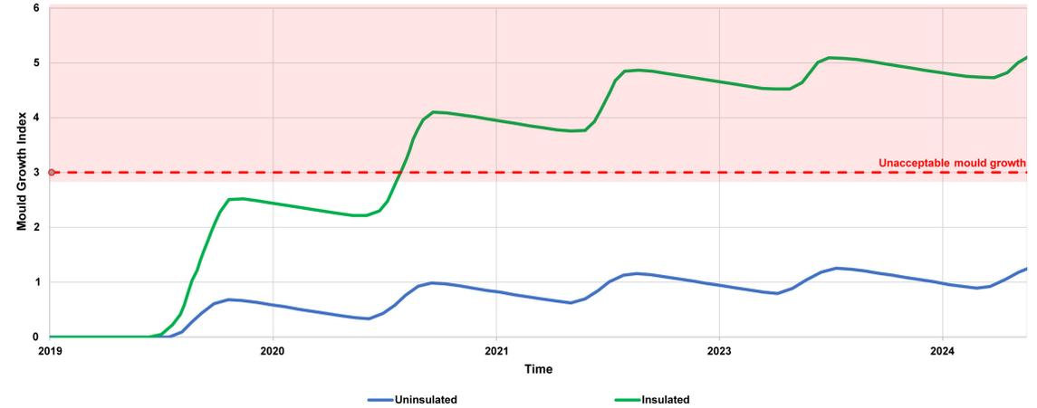
**Uninsulated** (the blue line) is the old-style roof with no insulation and good ventilation.
