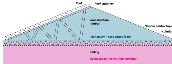
As the name indicates, a cold roof with a vapour control layer is a cold roof with a special membrane installed below the insulation at the ceiling line. A vapour control layer (V.C.L.) prevents water vapour molecules moving through it.
